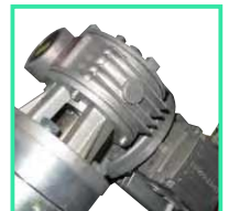
Motor with a gearbox of the pellet feeder
